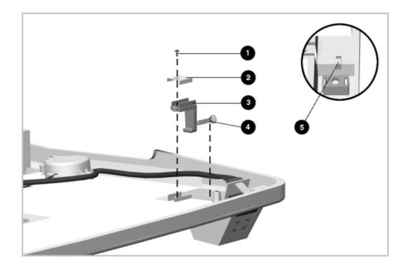
Figure 6-29. Removing the CPU Guide
